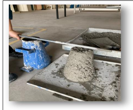
Figure 6. Using a slump test method.
