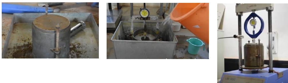
Figure 3: California Bearing test.
