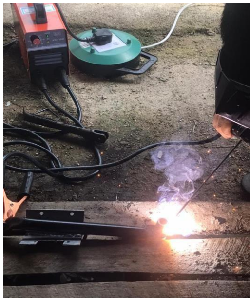
Figure 6: Welding process of the motorcycle side stand
