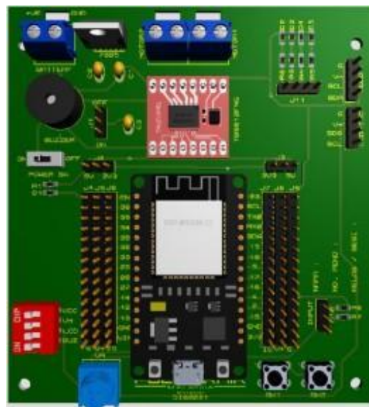
Rajah 5: Hasil Gambar 3D Kit Trainer ESP32
