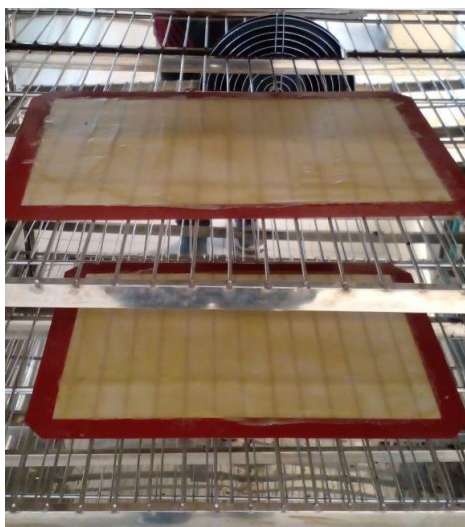
Figure 7: Drying in the drying oven for about 8 hours at 70°C
