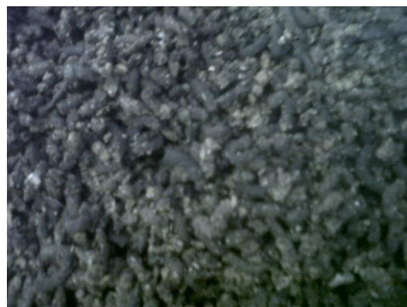
Figure 4. Pellet form for 3 mm mold size
