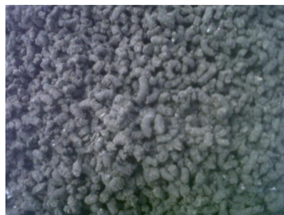
Figure 5. Pellet form for 4 mm mold size
