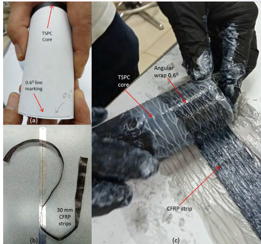
Figure 2. (a) Marking of 0.6^\circ angle line on TSPC column specimen. (b) 30 mm and 1250 mm in length of CFRP strip to wrap the TSPC column. (c) Wrapping process of CFRP strip onto TSPC column using epoxy Sikadur 330.
