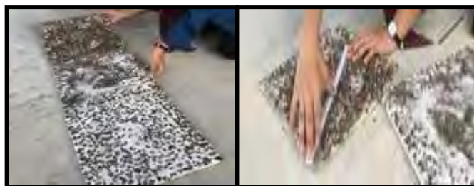
Figure 6. The sample of Cocolastic Tiles and measured the thickness
