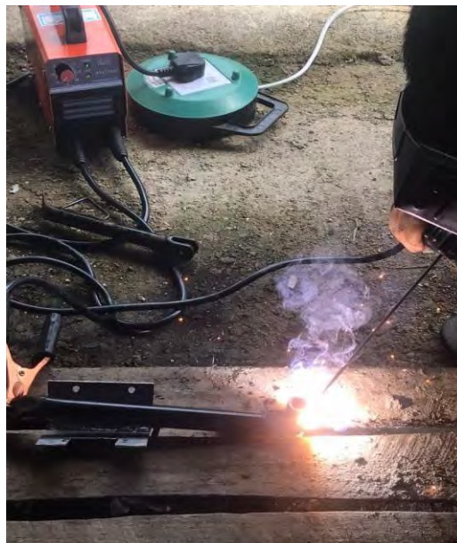
Figure 6: Welding process of the motorcycle side stand
