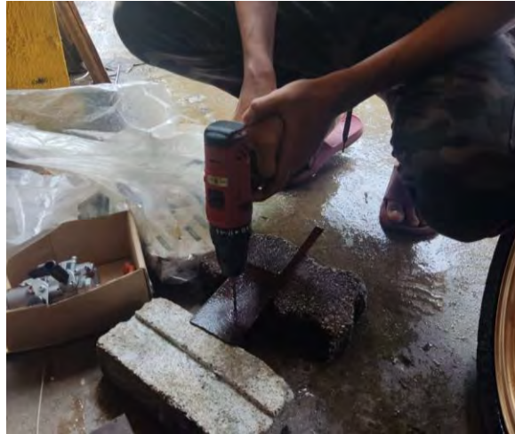
Figure 5: Process drill the frame of power side stand
