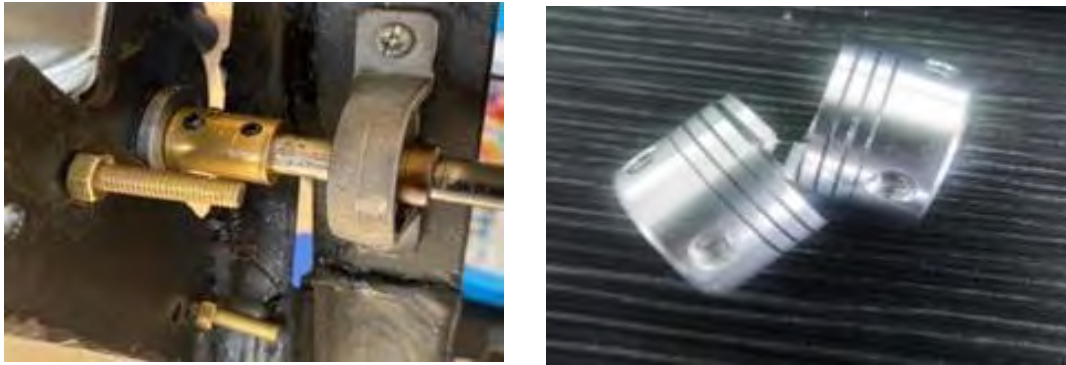
Figure 10: The rigid shaft coupler and flexible shaft coupler
