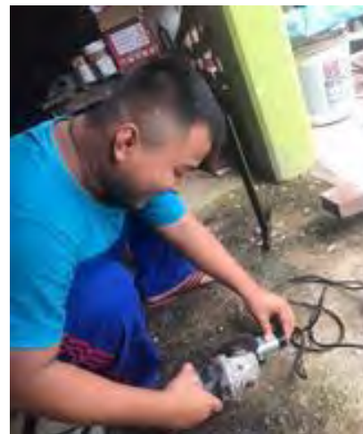
Figure 4: Proses cutting for assembly the frame of Power side Stand
