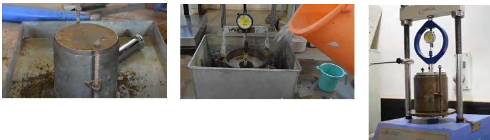
Figure 3: California Bearing test.
