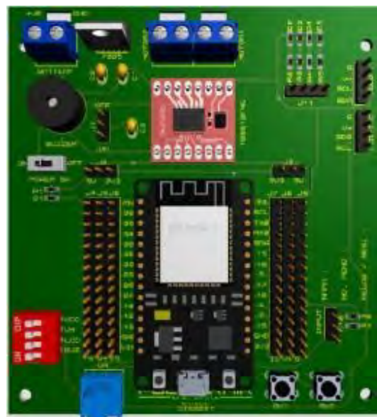
Rajah 5: Hasil Gambar 3D Kit Trainer ESP32
