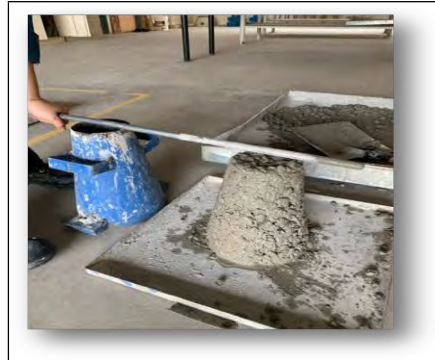
Figure 6. Using a slump test method.
